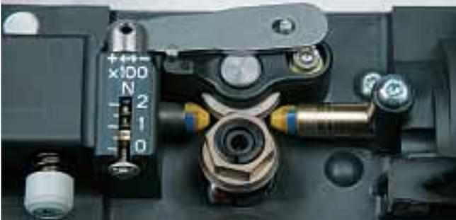
*The wire buffer decouples the front and rear wire-drives from one another and ensures smooth wire travel.*
