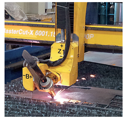
Universal carriage for combined technology - plasma and oxy-fuel as well as separate carriages for each technology or 3D tilting plasma tool station with ACTG
